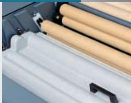
*A one-touch operated computer program allows automatic self-cleaning of the gum section.*
