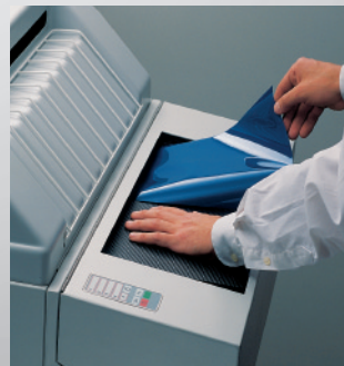
Sheet films can be processed by pressing downwards on the snap-down feed table.
